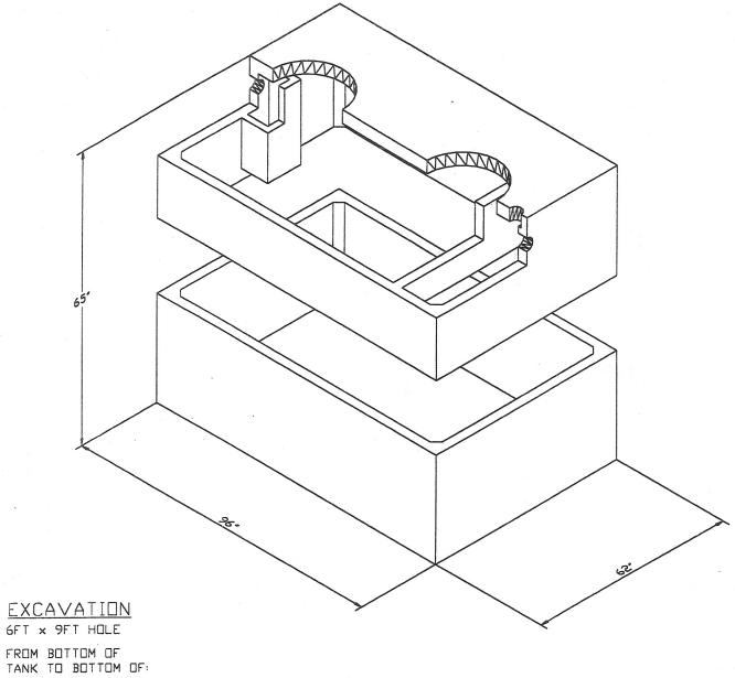
INLET PIPE - 55" **DUTLET PIPE - 52"**
